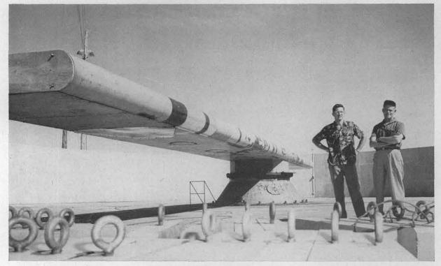
HUGE STEEL BOOM of the hydraulic centrifuge In the foreground are rows of heavy steel weights used dwarfs its operators, Milton Jones, left and Don McCoy. as counterbalances during Tech Area centrifuge tests.
